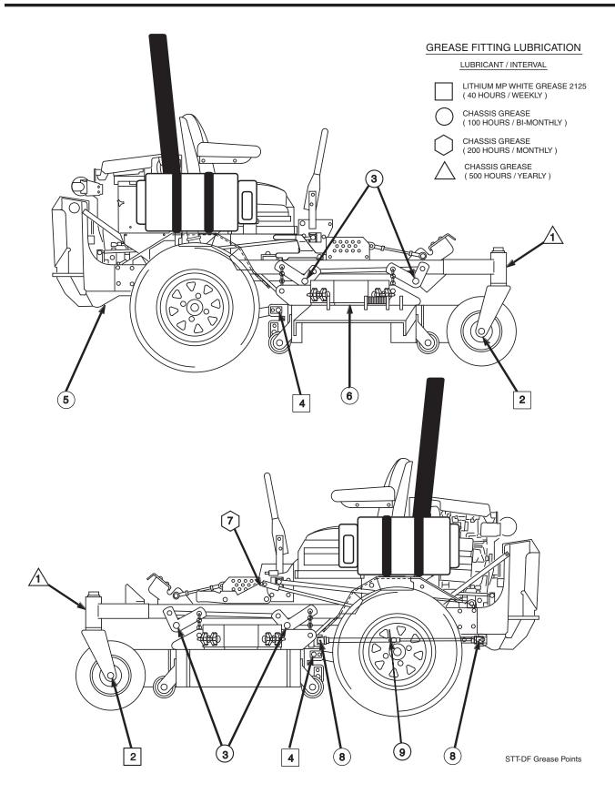
Figure 7-1. Lubrication Fitting Points
